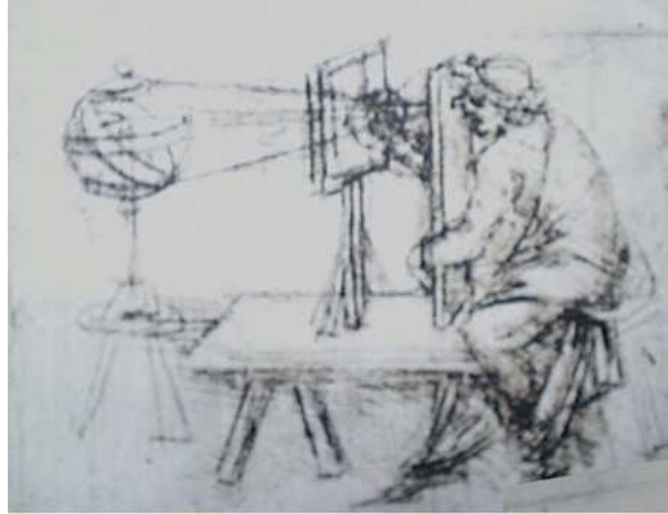
Figure 1. Drawing of a man using a perspectograph to draw an armillary sphere. Leonardo da Vinci ( Codex Atlanticus I, 5r; ~1480 )
